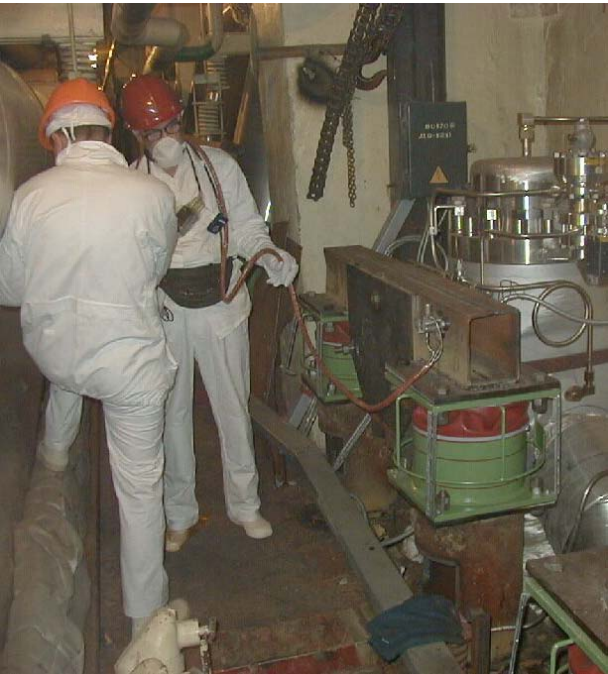
Figure 8. Vibration measurement on the Valve's 1211 damper plate.
