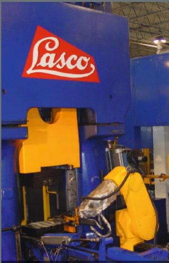
A Spring Supported Lasco Forging Hammer, Germany
