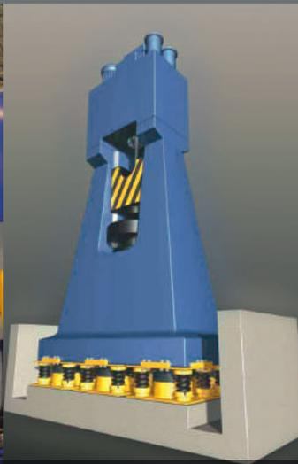
The principle of Direct Spring Support
