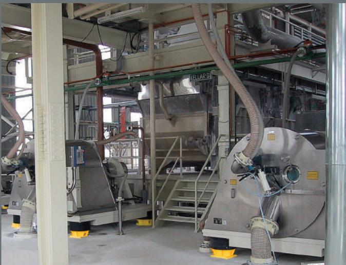
Vibration isolation of centrifuges, Germany
