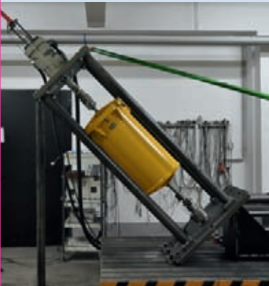
One Dimensional Prestressed Damping Device (PDD) in Test Stand
