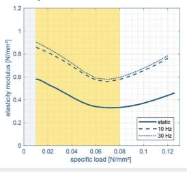
the perimeter surface. The greater the shape factor the stiffer the material. The shape factor varies from low density to compact. Therefore, for each product application a different shape factor yields a slightly different elastic curve. For this reason, our solutions are always project specific, resulting thus in a tailored elastic behavior depicted in he product data sheet and the quality assurance plan.
