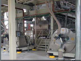
Vibration isolation of centrifuges, Germany
